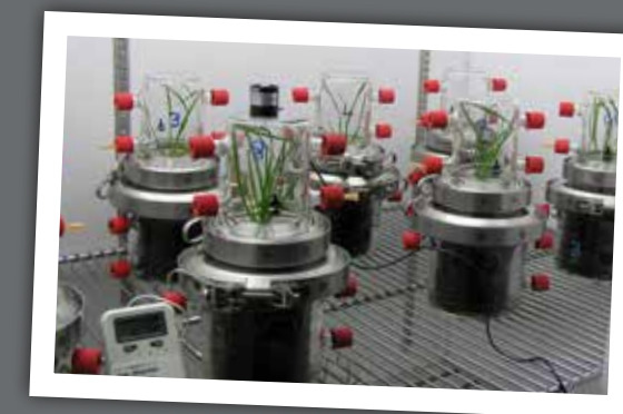
Nitrous oxide emission measurement units in a climate controlled plant growth cabinet
