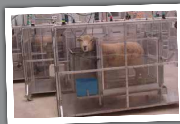
Individual sheep respirators for measuring the amount of methane produced
